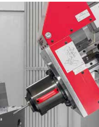
Compact and extremely rigid machine structure Developed using FEM (finite element method): In the TFZ series all components in the power transmission are optimized by static and dynamic considerations.
